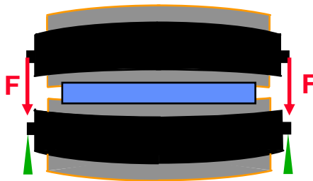
Fig. 2. In copiers and printers it is also important to have knowledge of the 3D-contact problem arising from the combination of the 2D-rolling contact and the bending of the rollers.
